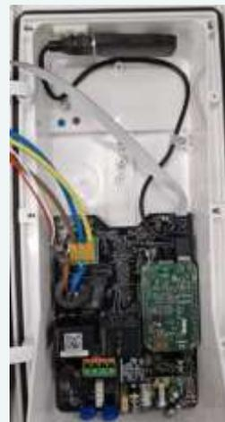
Figure 16: Smart PRO 4G Dongle Placement
