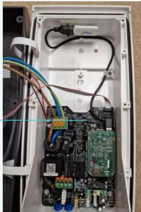
Figure 12: Smart PRO Dongle Placement
