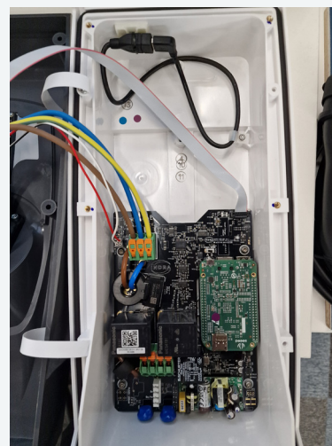
Figure 14a: Chargers with the USB cable pre-installed, connect the USB plug into the USB extension as per figure 14a
